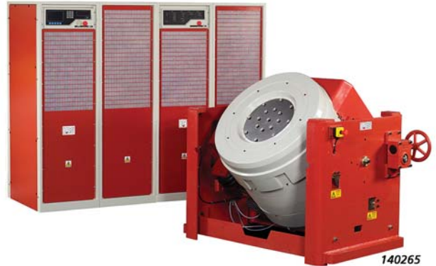
Fig. 3 SPA176K amplifier with integral FPS shown with a V9x shaker
